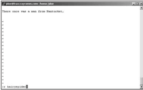
Figure 4.13 Reading an additional file into the current one can make your editing tasks much easier.
